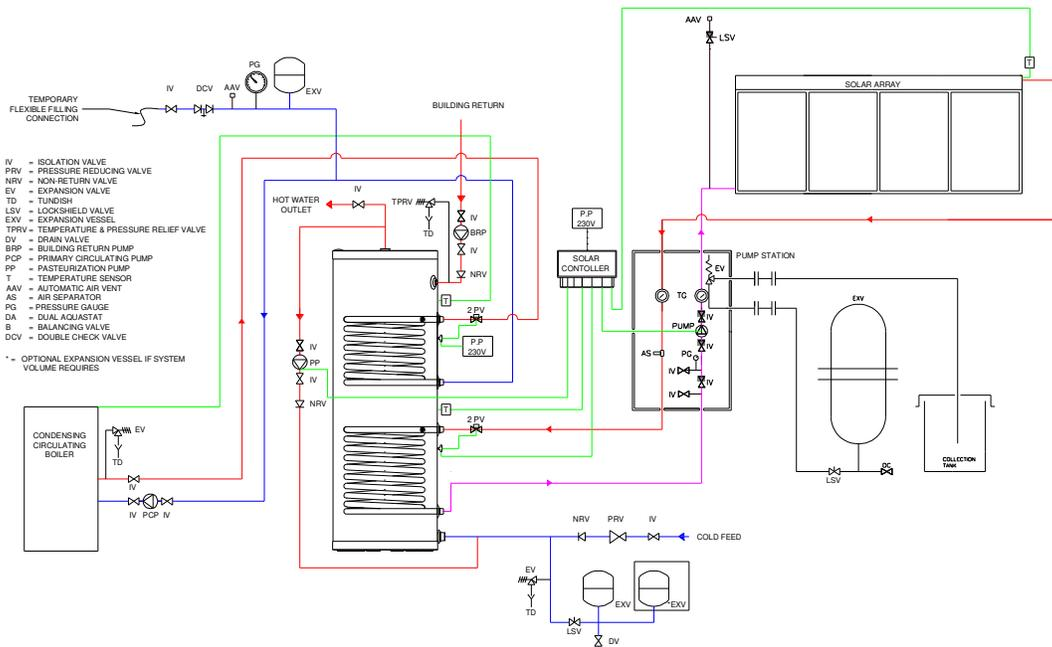
**5.3.3 RECOMMENDED PIPEWORK FOR SDT – SOLAR ARRAY, CIRCULATING BOILER**
