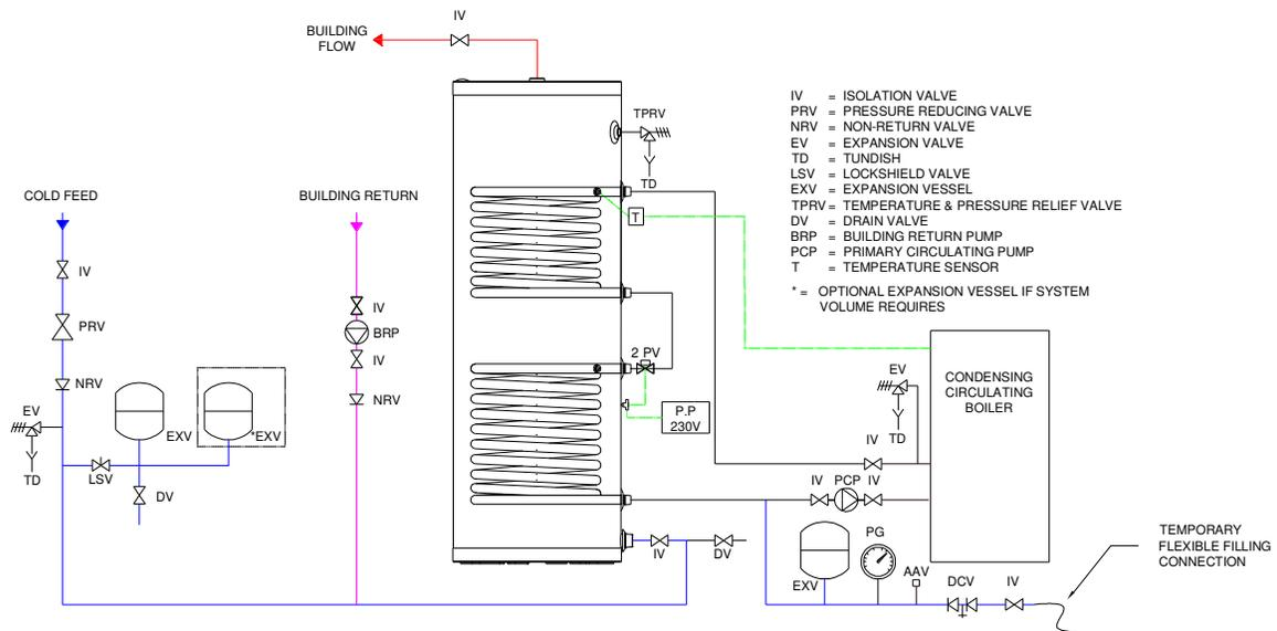
**5.3.4 RECOMMENDED PIPEWORK FOR SDT – CIRCULATING BOILER, HIGH RECOVERY RATES**
