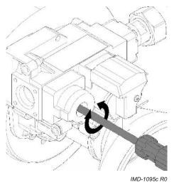
Fig. ECH 32-220 to 63-370 - CO<sub>2</sub> adjustment (partial load)
