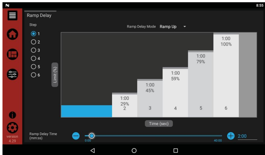
FIGURE 6 RAMP DELAY SCREEN
