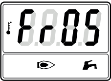
Fig. Frost protection is activated
