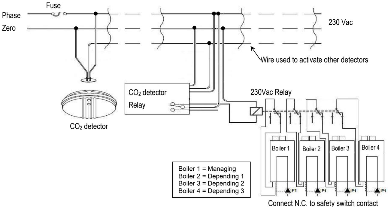
Use an extra 230V multipole relay (number of poles equal to number of boilers). In case of power failure on the CO alarm system and modules the boilers will shut down. Mount, install, test and maintain the CO detector according to the manufacturer's instructions. Test the system at least monthly, to ensure the boilers will switch off in case of a CO alarm.
