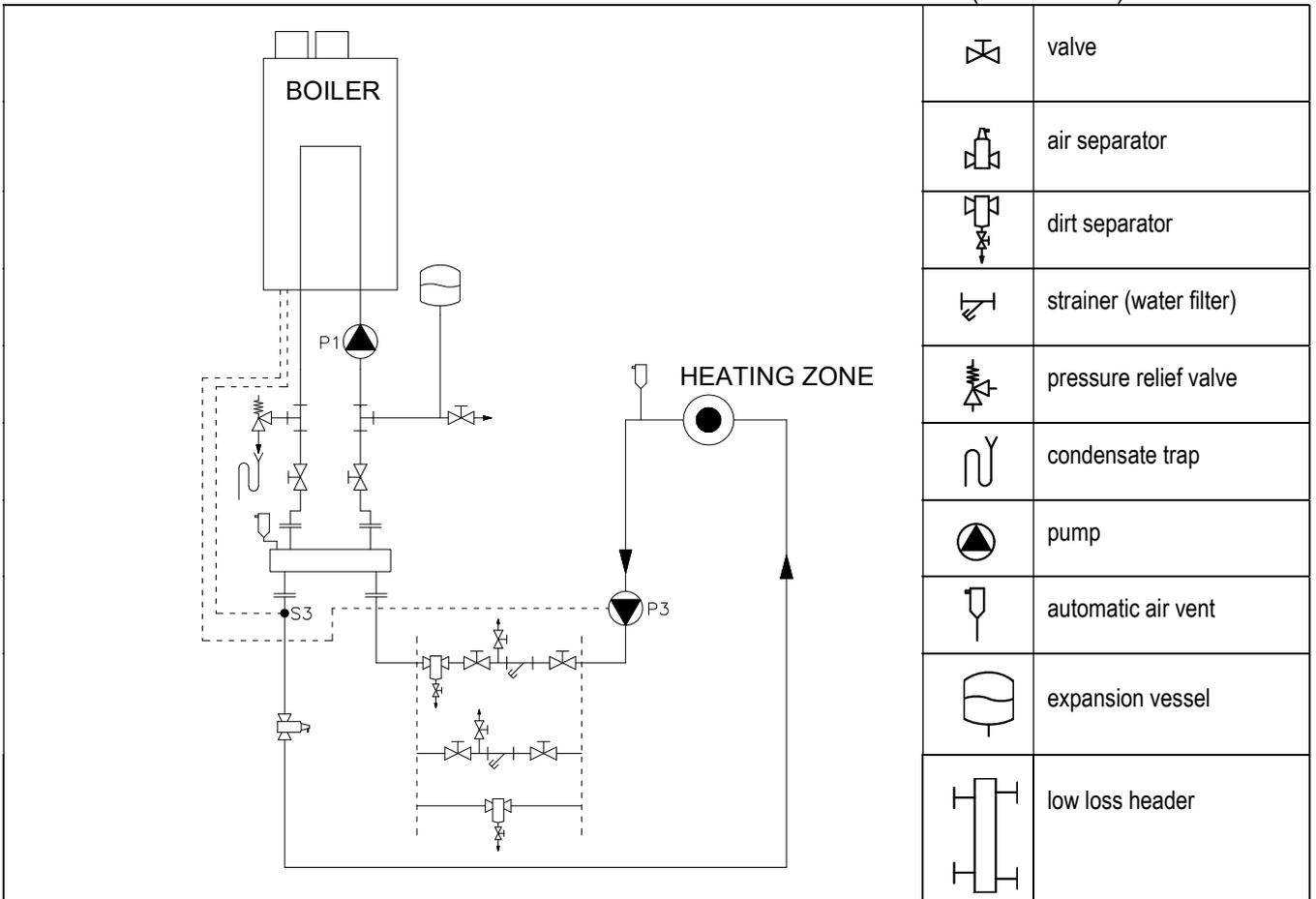
7.19.3 EXAMPLE OF A MULTIPLE BOILER HEATING CIRCUIT WITH LOW LOSS HEADER
