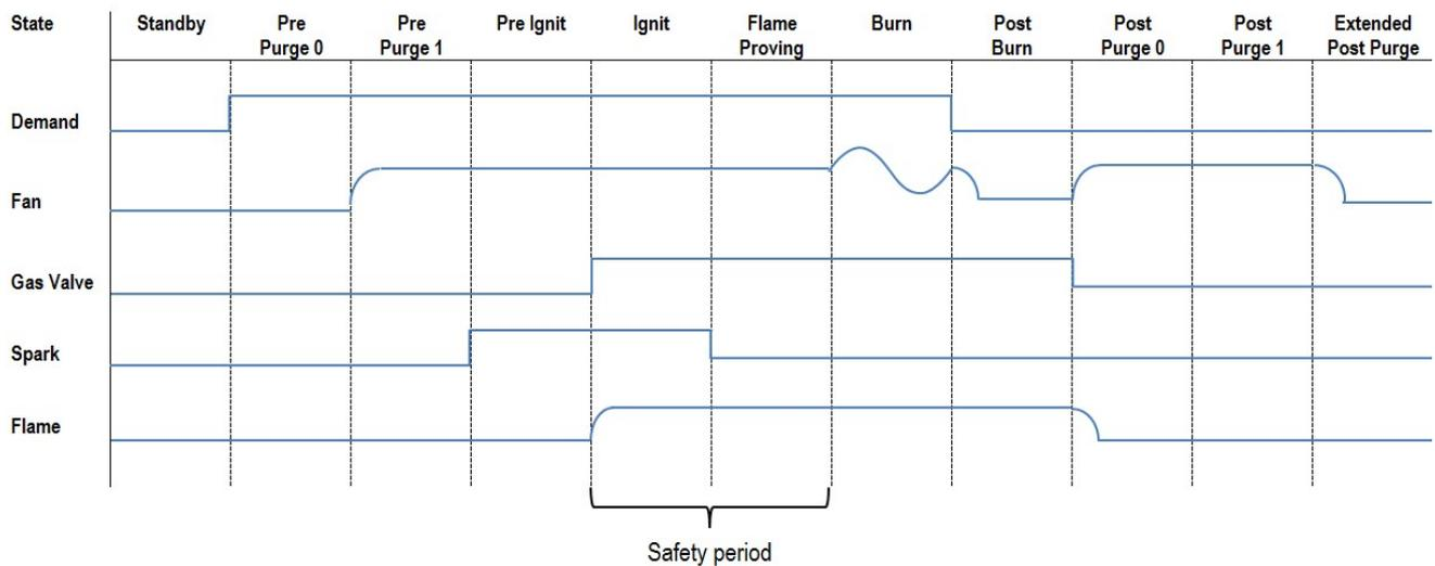
The table below shows the states of the burner ignition cycle, as shown in the diagram above:
