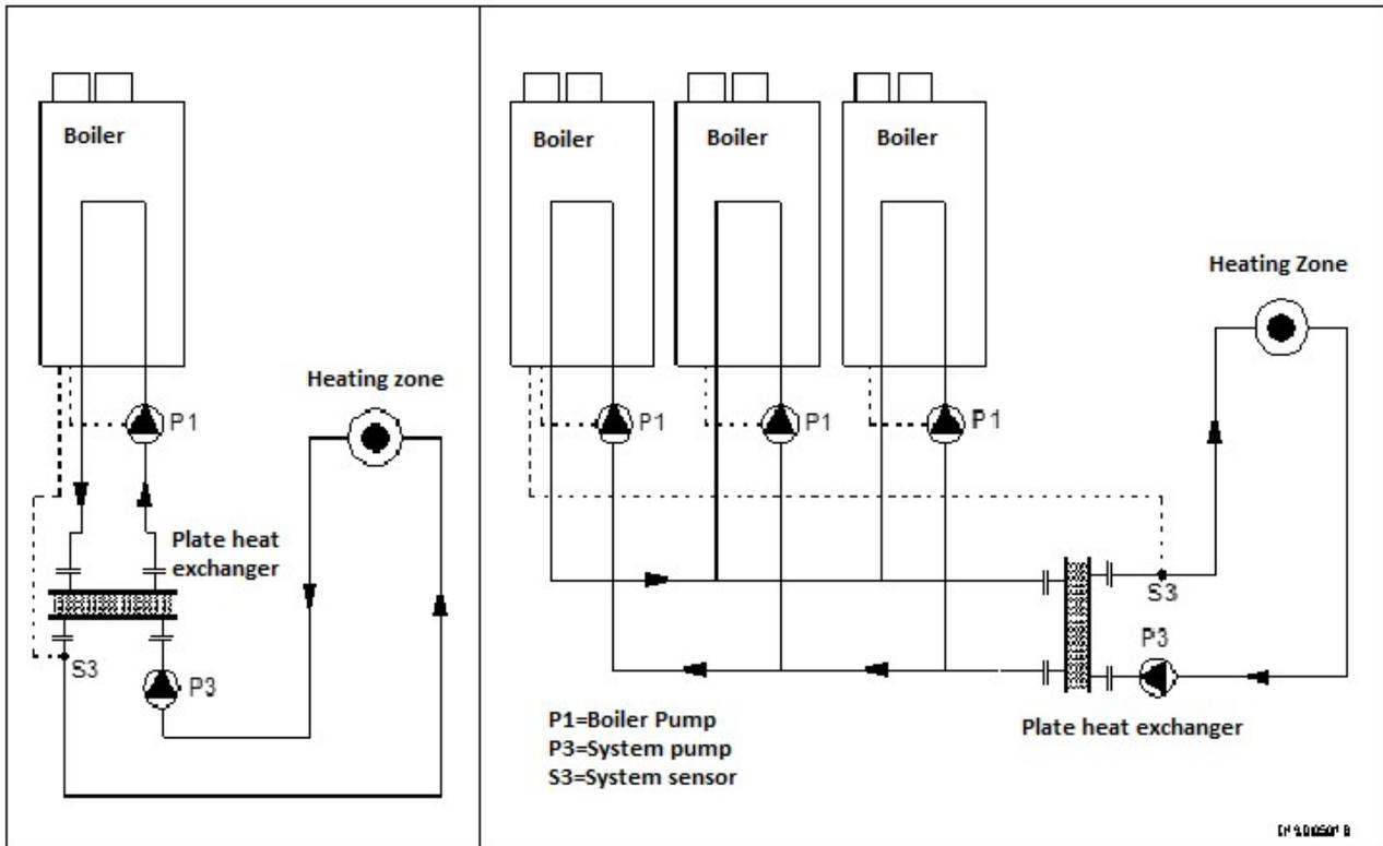
7.15.1 BOILER FITTED WITH PLATE HEAT EXCHANGER SIMPLE SCHEMATIC SHOWING CONCEPT
