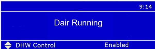
The "De-Air" sequence is a safety function that starts at every power-up and is used to remove the air from the heat exchanger. The De-Air sequence takes around 14 minutes to complete. It can be cancelled by pressing the Enter button for over 5 seconds. After completion or manual ending the "De-Air" sequence one of the following Status overview screens appears:
