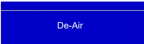
The "De-Air" sequence is a safety function that starts at every power-up and is used to remove the air from the heat exchanger. The De-Air sequence takes around 14 minutes to complete. It can be cancelled by pressing the Enter button for over 5 seconds.
