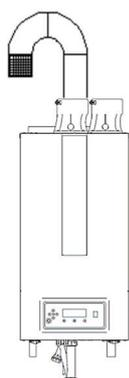
Boiler is IPX4D applying a dust filter or bird screen with two elbows and if necessary, a short straight pipe.
