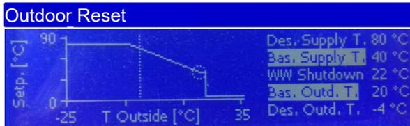
It now is possible to set the Outdoor reset curve by changing the parameters on the right hand of the screen.
