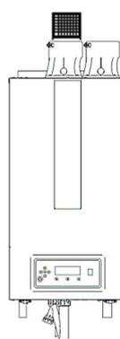
Boiler is IP20 applying a dust filter or bird screen only
