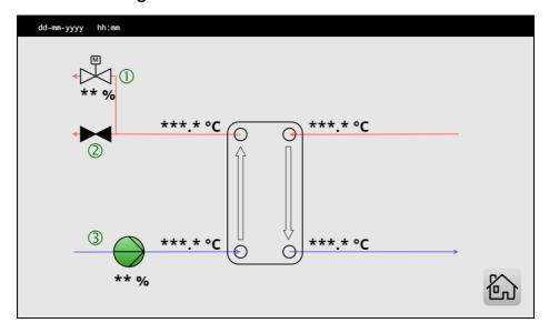
In the heat exchanger screen the user can find information about the heat exchanger temperatures, the transfer loop pump (TL02.CP01) and information about the valve statuses which regulate one-pass (OP) or multi-pass (MP) behaviour (where applicable).
