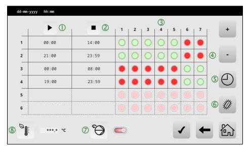
An ECO program can be programmed to temporary increase or decrease water temperatures. Up to six blocks of times can be defined.
