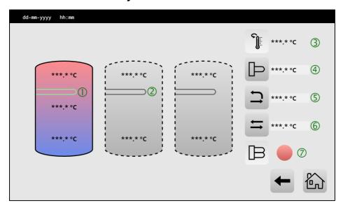
In the domestic hot water (DHW) screen several parameters of the DHW system can be seen and set.
