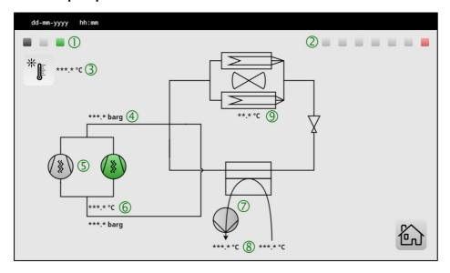
The heat pump information screen gives the user info about the heat pump system. The user can switch between heat pumps by clicking on the respective square (1, 2). A green square indicates a running unit, a grey square indicates a stand-by unit and a red square indicates a unit in alarm mode. The status of components is shown in green (in operation) or grey (stand-by)
