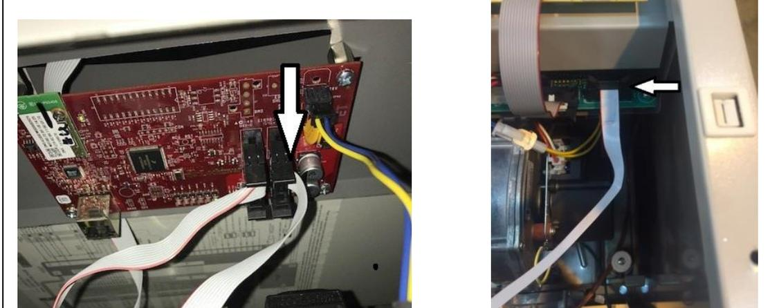
13. Disconnect the power supply connection from the transformer to the main control PCB.
