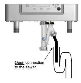
The condensate drain is placed at the centre and at the bottom of the boiler and has a 19 mm hose discharge. Connect this flexible hose to the sewer system.
