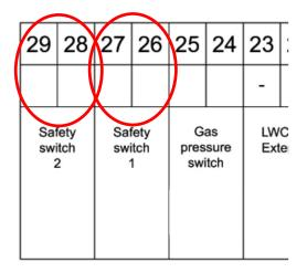
Low voltage connections EFB boiler.
