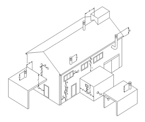
9.3.1 FLUE TERMINAL POSITIONS Use in conjunction with table 9.3.2
