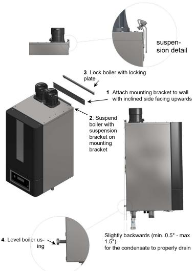
Lock the mounting bracket with the security cover before making any other connections to the boiler. This security cover will prevent the boiler from falling off the bracket. Do not use excessive force during the mounting of the boiler connections.
