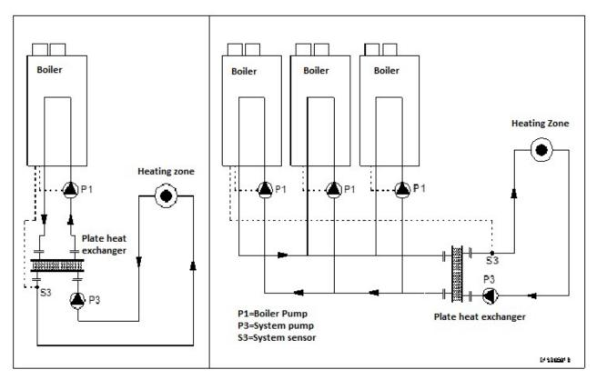
7.15.1 BOILER FITTED WITH PLATE HEAT EXCHANGER SIMPLE SCHEMATIC SHOWING CONCEPT
