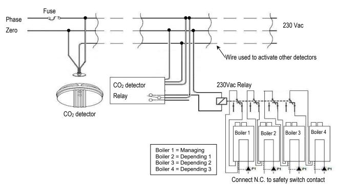
Use an extra 230V multipole relay (number of poles equal to number of boilers). In case of power failure on the CO alarm system and modules the boilers will shut down. Mount, install, test and maintain the CO detector according to the manufacturer's instructions. Test the system at least monthly, to ensure the boilers will switch off in case of a CO alarm.
