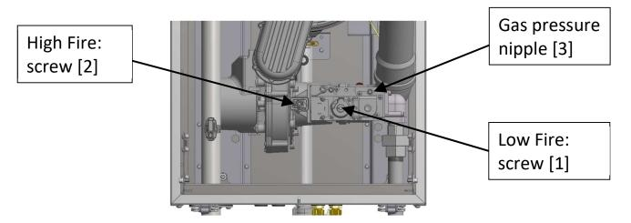
High Fire: venturi adjustment screw: use hex key 4 mm (5/32 Allen wrench)
