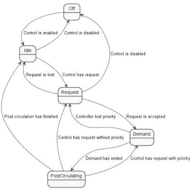
Dependent on the required functions of the appliance and connected sensors and components, several operation modes for Central Heating (CH) and Domestic Hot Water (DHW) can be selected, which are described hereafter.
