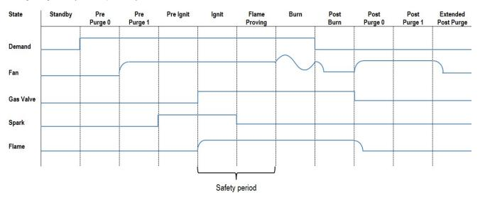
The table below shows the states of the burner ignition cycle, as shown in the diagram above:
