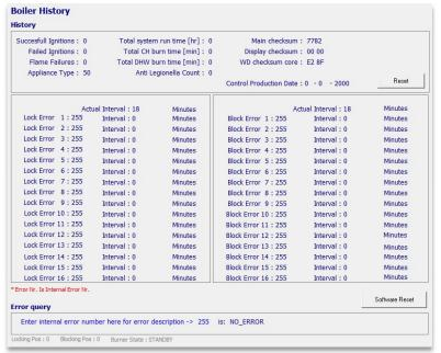
The last 15 lockout and 15 blocking errors are stored in the boiler controller. This boiler history can be shown via the Boiler History screen via the installer boiler status menu in one of the advanced displays.
