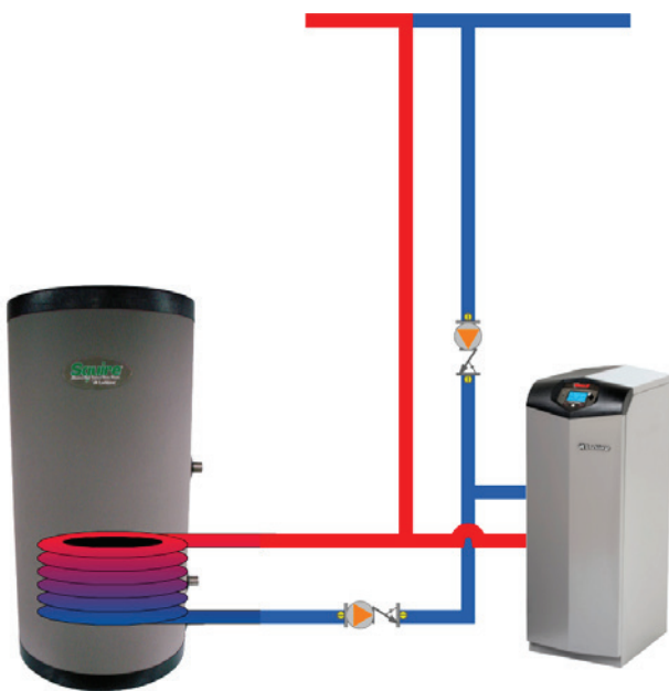
Lochinvar Herald boiler with Squire stainless SIT single coil Indirect water heater
