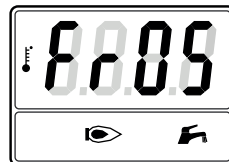
Fig. Frost protection is activated
