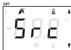
Fig. Service required display
